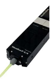
The 2-component dosing system ViscoDuo-P 4/4 is a valveless, static mixing head with dispensers located directly in front of the mixer. Especially developed for simplified cleaning (Easy Clean) and maintenance. In the mixing head no valves are required. The components to be mixed are dosed by volume only and with no dead space into the static mixer.
