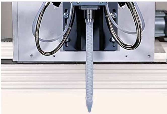
Automatic production application with the MK 20/21 mixing head
