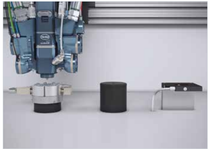
Left Side: The pneumatic AIR-CLEAN nozzle cleaning system cleans the mixing head nozzle by means of compressed air. Middle: Device for high-pressure water rinsing and filling shot station. Right Side: The NOZZLE-CONTROL laser-based nozzle measuring unit checks that the dosing nozzle is in the correct position and there is no contamination.
