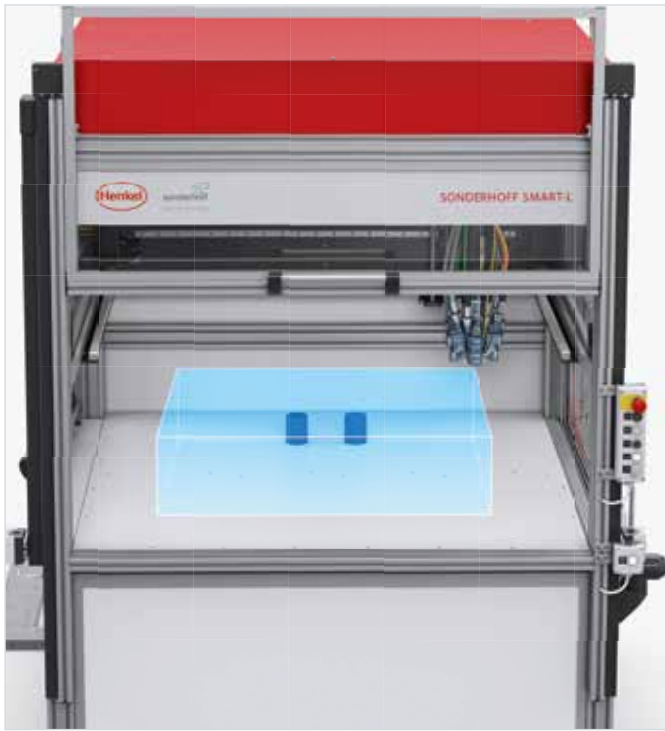
Travel range in the SONDERHOFF SMART-L dosing cell: 1,000 x 800 x 250 mm (x/y/z)
