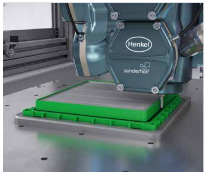
FERMAPOR K31 sealing foam dosed application with the MK 800 PRO mixing head for bonding the filter frame
