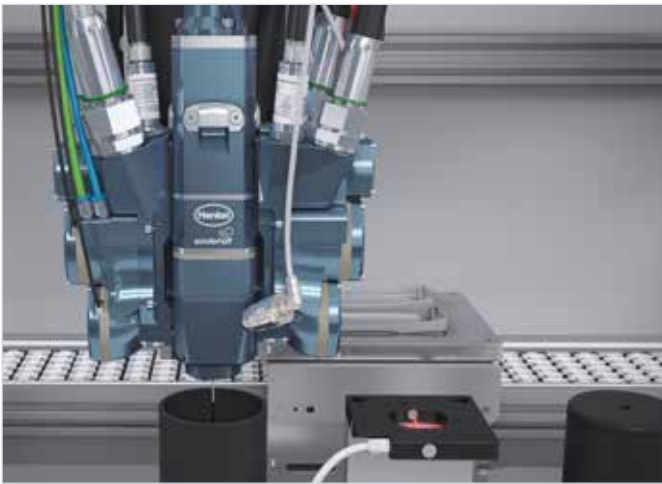
The MK 800 PRO mixing head is in the filling shot position.
