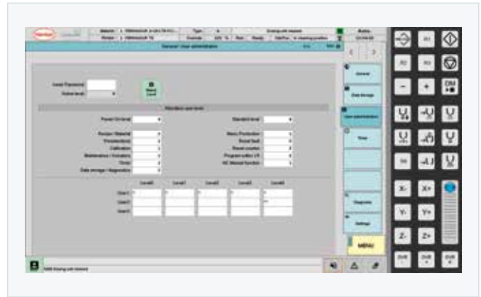
Password: User management for three users with the possibility to configure differentiated access via password levels (0-4)
