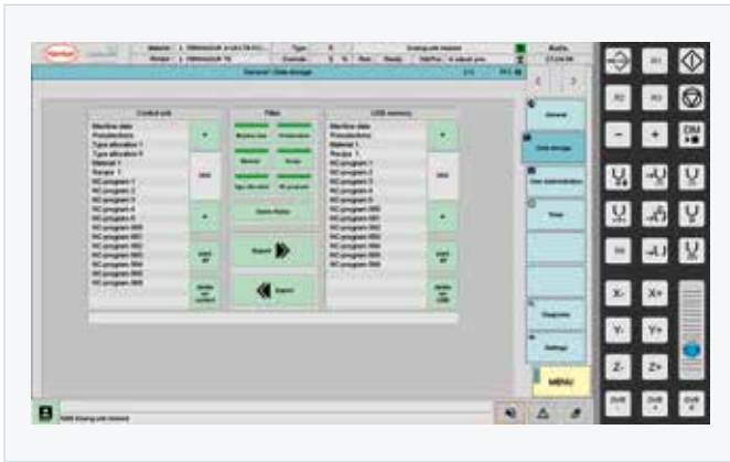
Data backup: Allows selective selection of machine data, presets, type assignment, material, recipe and NC program to be saved
