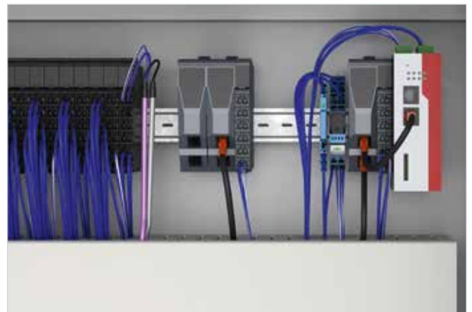
VPN router for remote maintenance (remote collaboration)
