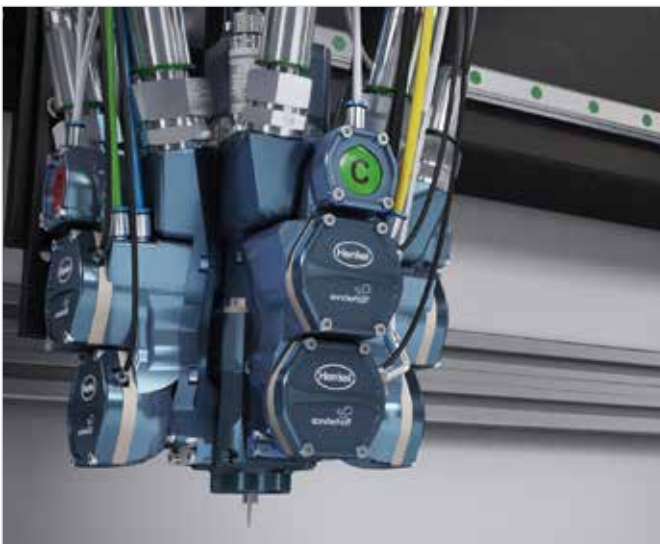
MK 800 PRO precision mixing head for 3 material components
