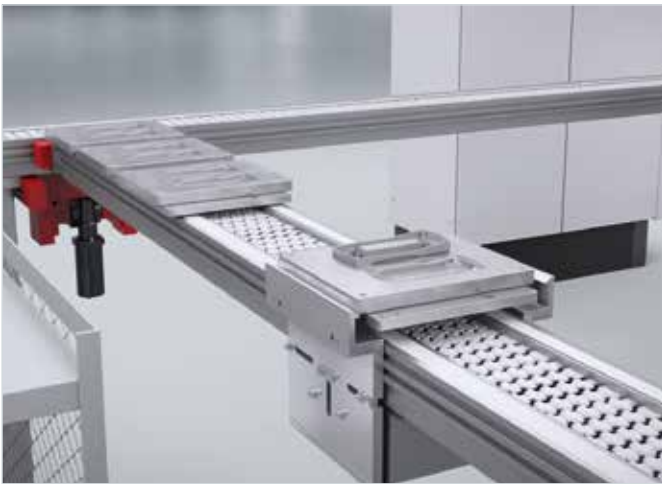
Loading of workpiece carriers and feeding on the conveyor belt to the dosing cell
