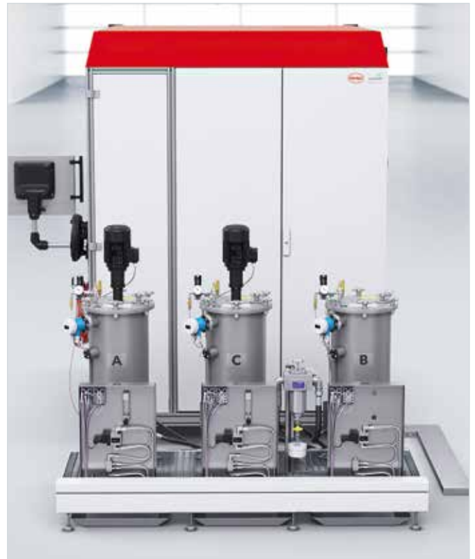
Dosing machine cabinet integrated in the rear of the cell with hinged doors and material pressure tank (24 l or 44 l, single-walled or double-walled) on grating platform with adjustable leveling feet and drip tray
