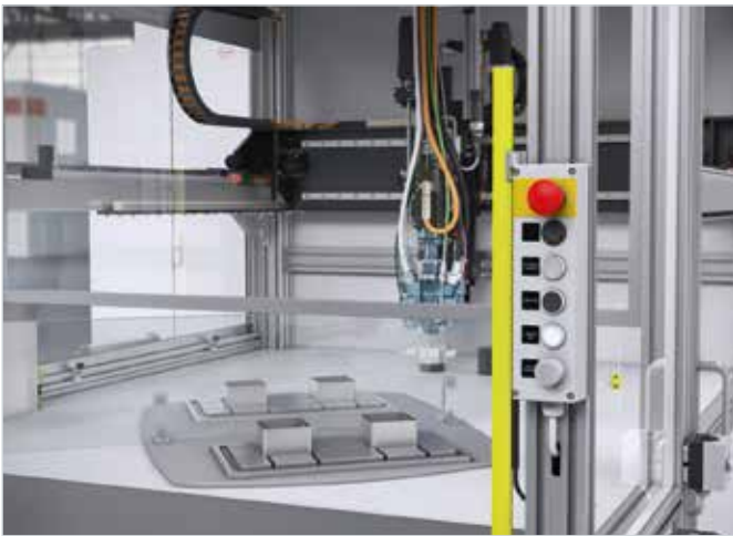
Rotary indexing table rotates 180° into the dosing position for contour-accurate movement of the component for material application
