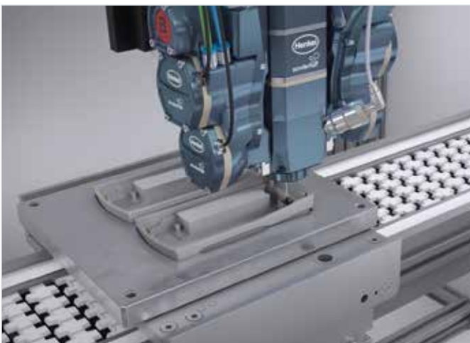
The CNC-guided mixing head precisely positions itself above the component and doses the potting compound.
