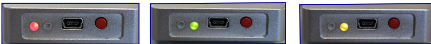
Different modes (Stop, Run, Pause) are indicated by the color of the LED
