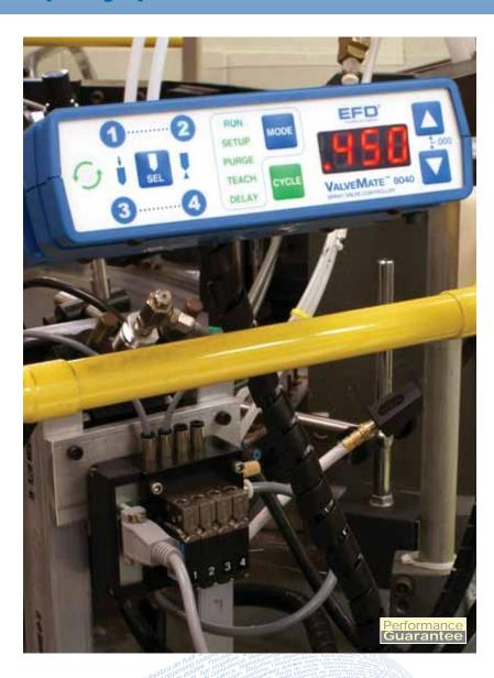
Spray pattern is defined through a combination of fluid pressure, valve stroke and valve open time, with valve open time providing the greatest control over the volume of fluid sprayed.
