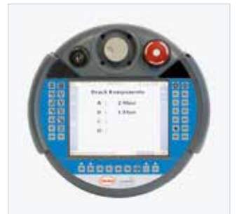
Basic equipment: multifunctional mobile panel SONDERHOFF MP (6.5")
