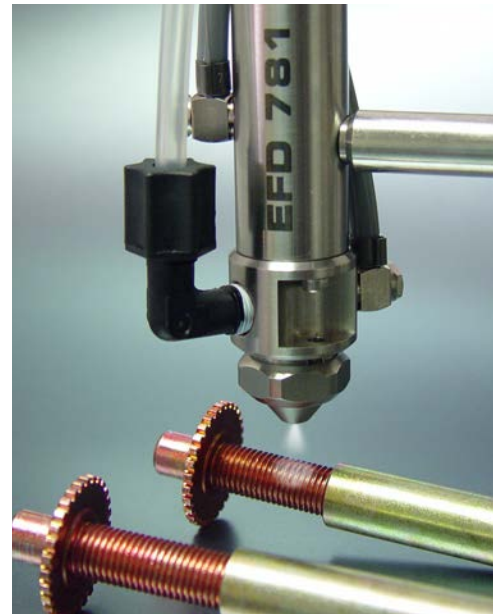
781S sprays lubricant on automotive brake adjusters.
